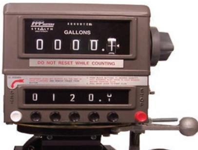
Register stack attaches to the RAD with 4 screws, 2 front and 2 rear.
